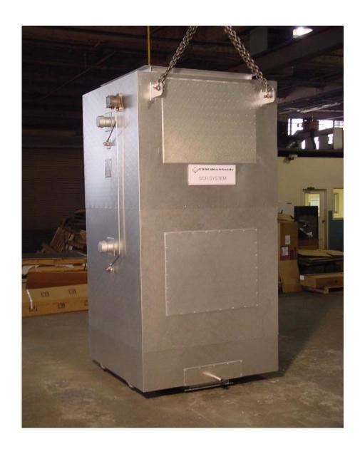
5 PPMV NOx Emissions Achieved in the Exhause of an Industrial Process Boiler by this CSM SCR System Operating in Anaheim, CA within the South Coast AQMD.
