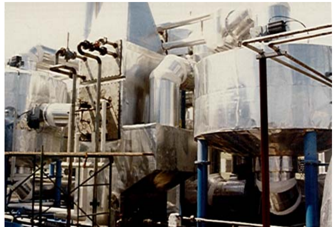
RAYSORB Solvent Recovery System recovers 300 lb/hr. of Methylene Chloride/ Ethanol solvent mixture
