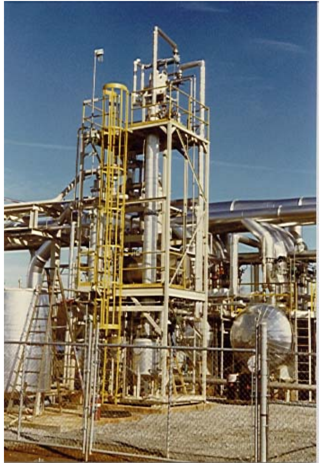
900 lb/hr. Isopropyl Acetate/Isopropanol package distillation system, 316 SS with automatic stripping and process heat recovery.
