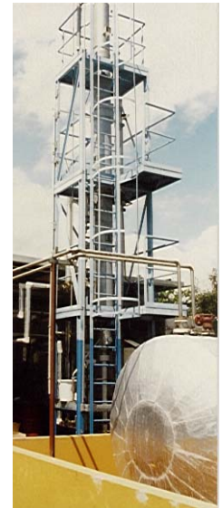
900 lb/hr. Isopropyl Acetate/Isopropanol package distillation system, 316 SS with automatic stripping and process heat recovery.
